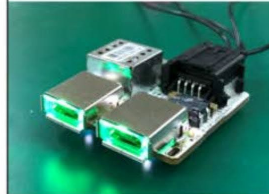
Charging Module: USB A / USB C with built-in Light guide (Tandem)
